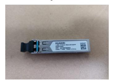
The Huawei MXPD-243S is a reliable and high-performance 1.25G SFP (Small Form-Factor Pluggable) optical transceiver, designed to deliver seamless Gigabit Ethernet and Fast Ethernet connectivity over singlemode fiber. With a 1310nm wavelength and a maximum transmission distance of 10km, this SFP module is the ideal choice for ISPs, enterprises, and data centers in Kenya and East Africa.
